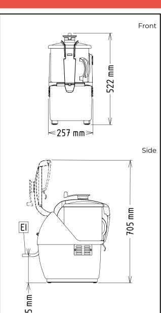
Electric Supply voltage: 200-240 V/1N ph/50/60 Hz Electrical power, max: 1.5 kW 1.5 kW **Total Watts:** Capacity: Performance (up to): 3.5 kg/Cycle **Capacity:** 7 litres Key Information: External dimensions, Width: 256 mm External dimensions, 422 mm Depth: External dimensions, Height: 522 mm **Shipping weight:** 27 kg
